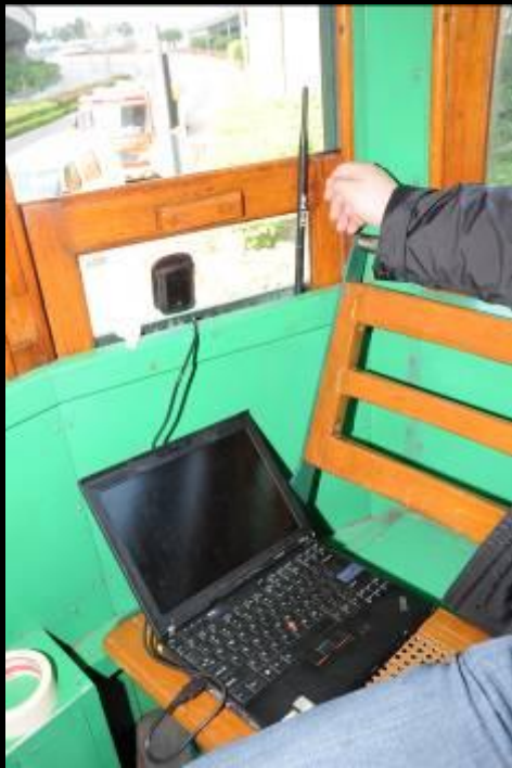
Standard War Driving Equipment: Notebook, Antenna, and GPS device
